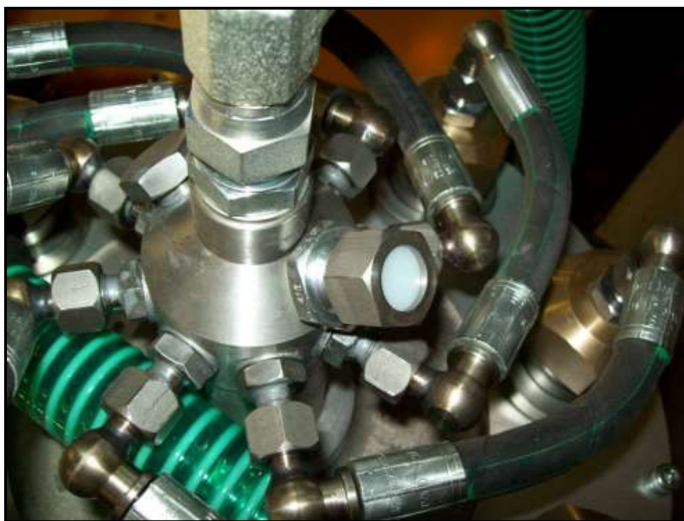
Fig. 6.2 Burst disc holder showing 'white' burst disc
