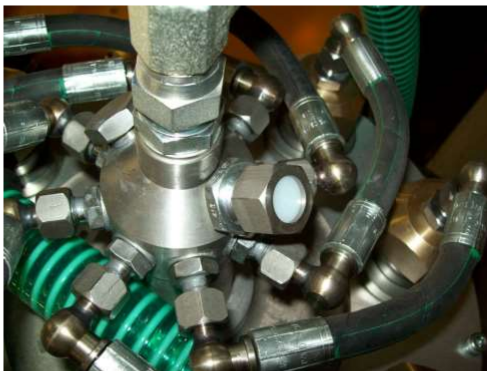
Fig. 6.2 Burst disc holder showing 'white' burst disc
