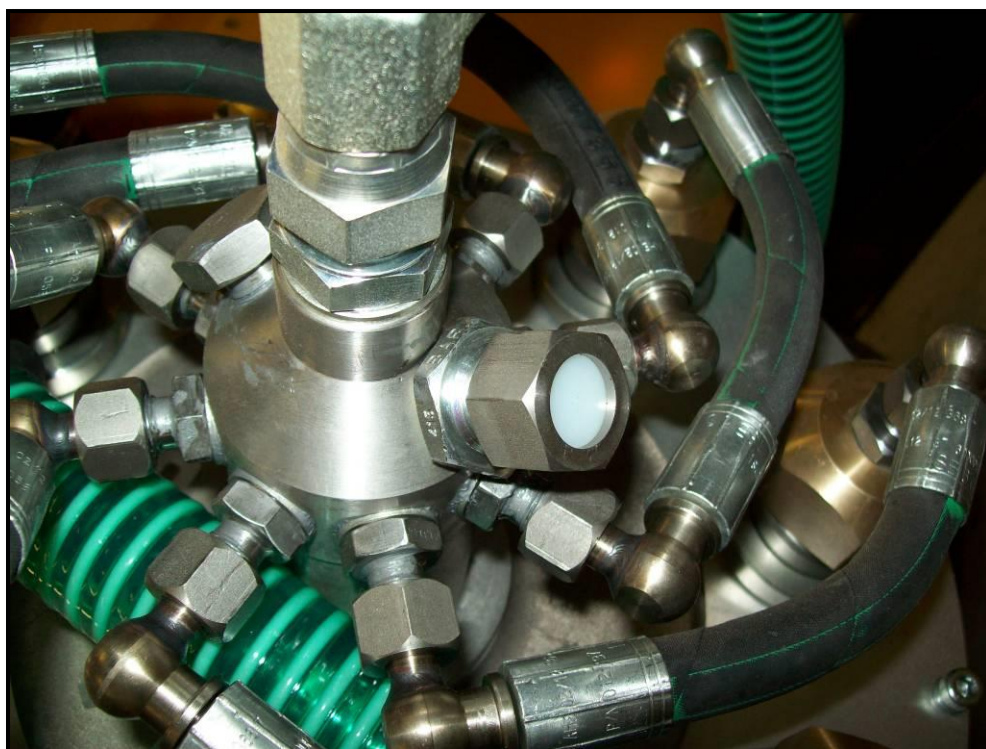
Fig. 6.2 Burst disc holder showing 'white' burst disc
