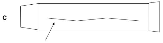
Shear through wall of diaphragm
