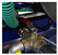
2. Put the Tank Drain valve (Red) into the DRAIN position and drain the water tanks. When the tanks have drained move the valve to the SHUT OFF position.
