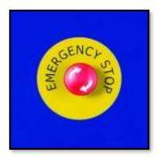
At any time during the starting procedure, or during normal jetting operations, an emergency shutdown can be achieved by switching off the engine with the key or pressing the E/Stop button.
