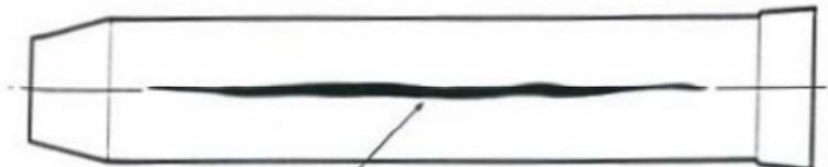
SHEAR THROUGH WALL OF DIAPHRAGM. CAUSED BY FATIGUE FROM EXCESSIVE RUNNING HOURS.
