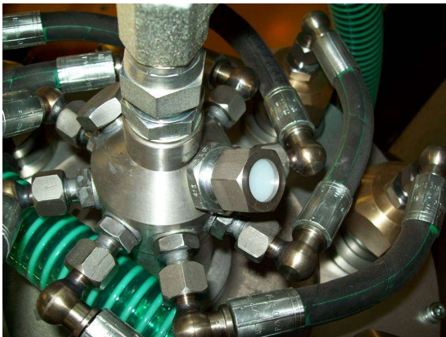
(Burst disc holder showing “White” burst disc)
