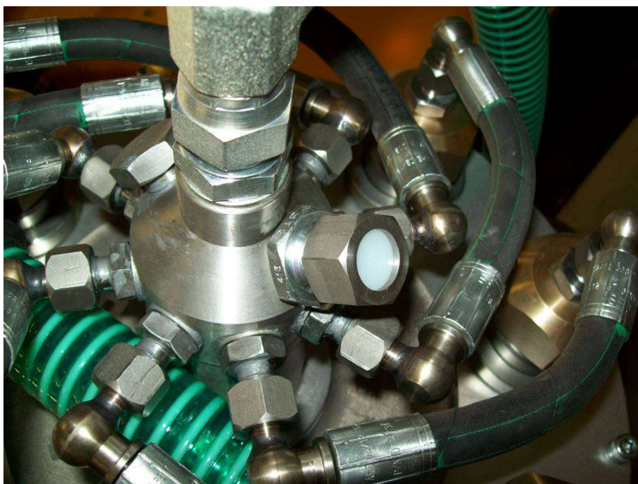
(Burst disc holder showing “White” burst disc)
