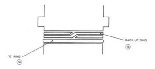
Fig 4.2 Inlet Valve Seat – Back Up Ring and 'O' Ring Fitting
