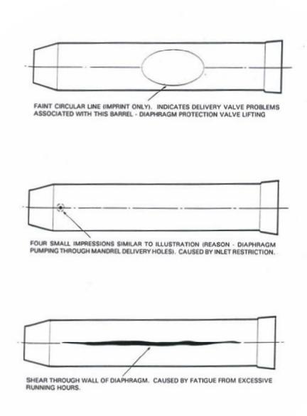
Fig 3.2 Pump Fault Finding – Diaphragm Failure and Indication of Other Problems
