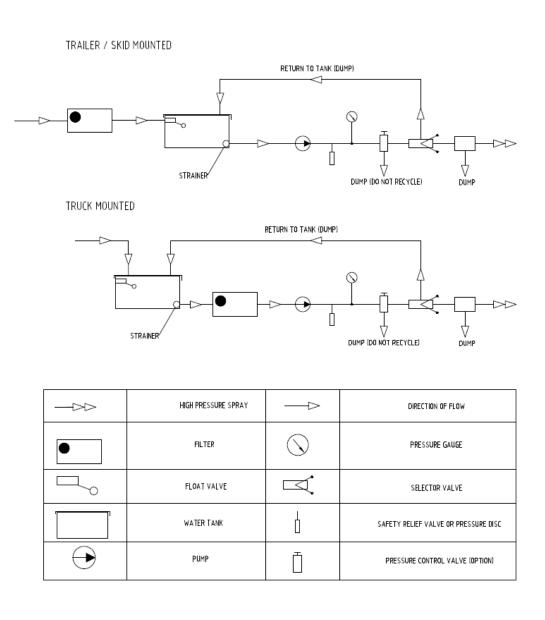
Fig 2.1 Pump Installation – Water Circuit Layout
