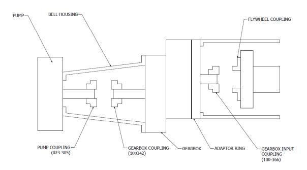
Fig 2.2 Pump Installation – Prime Movers/Gearbox/Pump Coupling Arrangements
