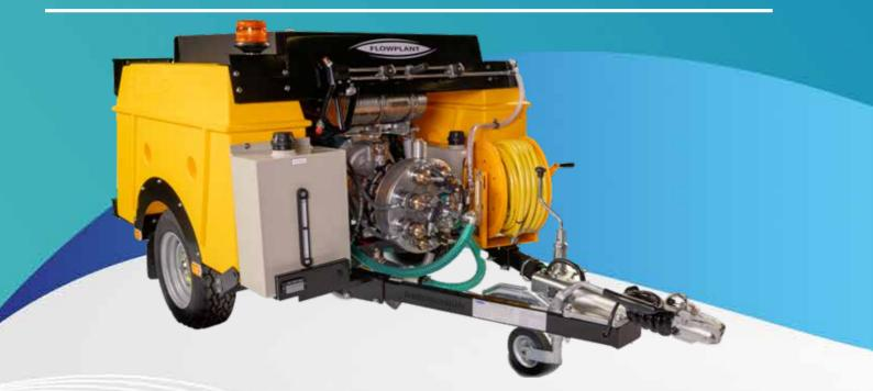
...The Jump Jet pulses the desilting hose reducing the friction of the hose against the wall of the cable duct. This allows the desilting nozzle to travel long distances into the duct, unblocking as it goes.
