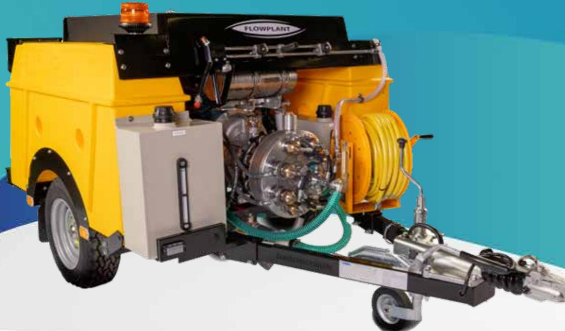
...The Jump Jet pulses the desilting hose reducing the friction of the hose against the wall of the cable duct. This allows the desilting nozzle to travel long distances into the duct, unblocking as it goes.
