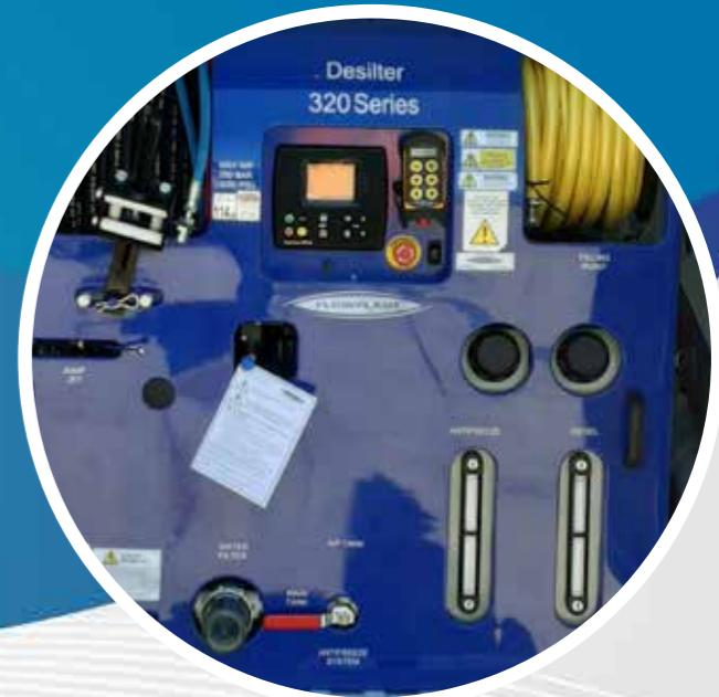
The solution comes in the form of a pulsing water jet created by the Harben Jump Jet™ system. The pulsations flex a special lightweight hose helping it to travel hundreds of meters into the duct, clearing silt as it goes. Unlike any other cleaning system the Harben Desilter works at pressures which do not risk cable damage but unbelievably it can still clean vast lengths, with a small amount of water.
