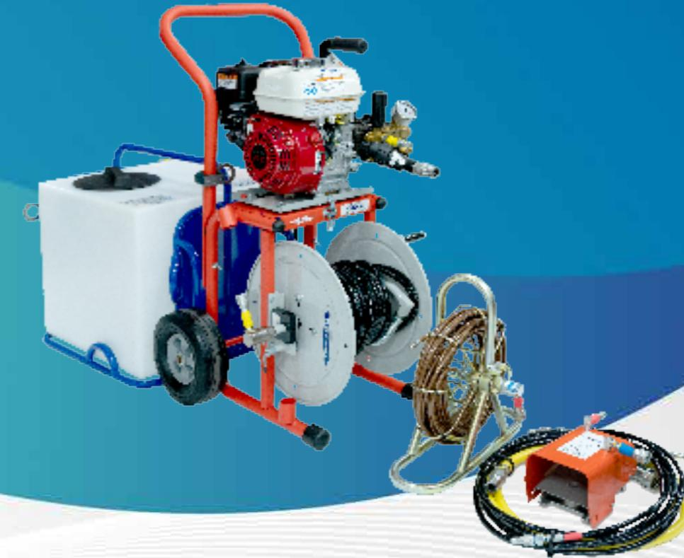
The Mini cable duct Desilter has a removable hose reel, safety foot control pedal and 140 litre water tank. All the items are modular and can be ready to use within minutes of arriving on site. They can be transported strapped together or as separately, depending on the space available in your vehicle. The mini desilter is supplied as standard with all the necessary accessories and is purchased as a complete system.
