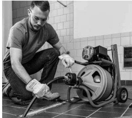
Figure 16 – Using Machine with Guide Hose
