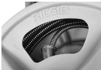
Figure 18 – Coil Cable Into Drum As Shown
