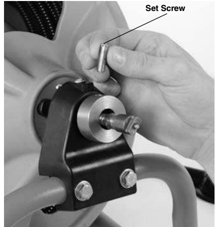
Figure 3 – Remove and discard the Cable Lock Set Screw
