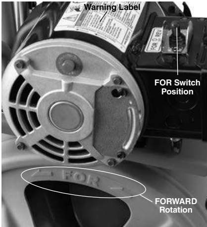
Figure 8 – Proper Drum Rotation (FOR Switch Position)
