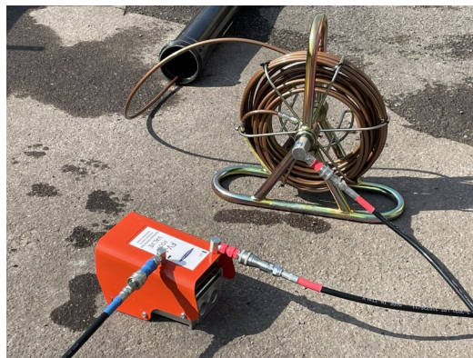
Desilter Hose Reel with 20m of micro bore desilter hose
