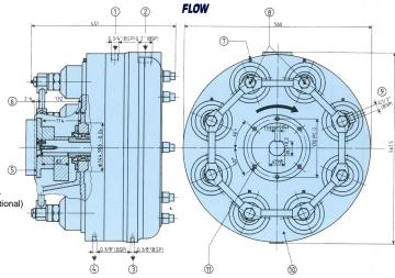
Dimensions in mm are identical for all pump models i.e. 4 & 8 cylinders.
