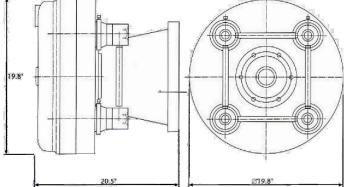
Note: The "Hi-Q" pump is suitable for gearbox, direct and hydraulic drive systems. Details of individual mounting methods are available upon request.
